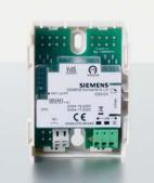
Input/output modules further increase safety and security. With the input modules FDCI221/FDCI222, you can monitor the status of doors, ventilation or sprinklers. The input/ output modules FDCIO221/FDCIO222 enable decentralized control of fire doors and plant. The "transponder" FDCIO223 enables a monitored connection of conventional detector lines, alarm signaling devices, and devices in explosion-protected zones.
